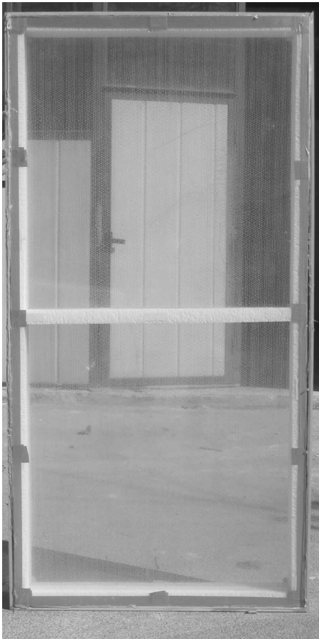
FIG. 8. Prototype of the transparent sound-absorbing panel employed for the reverberation room tests. Panel dimensions are 1.04 \times 2.05 m.
