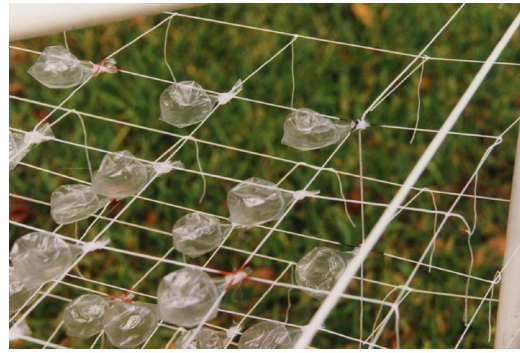
FIG. 2. (Color online) Detail of the bubble school, showing supporting multifilament netting and bubbles glued into position.
