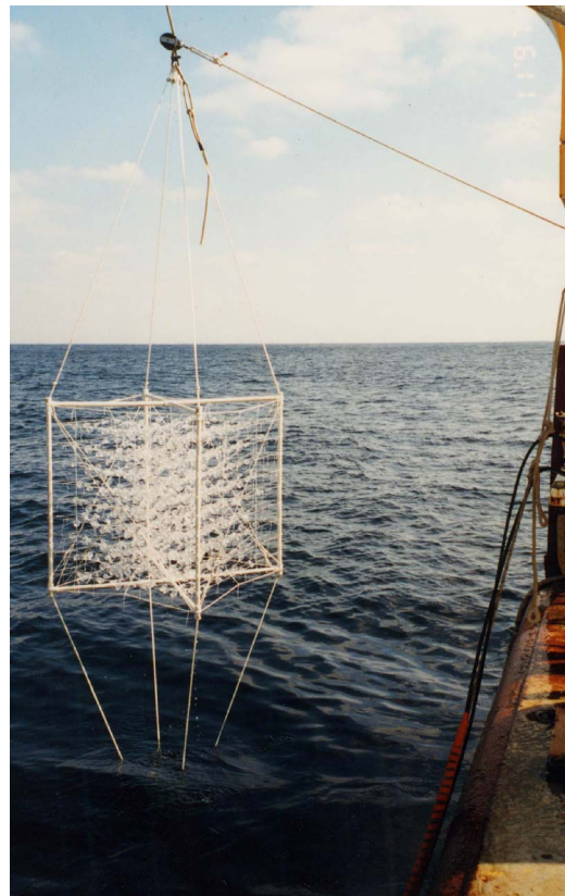
FIG. 3. (Color online) Dense bubble school being retrieved at sea. The 9×9×9 array of bubbles, and the PVC frame, are clearly displayed.
